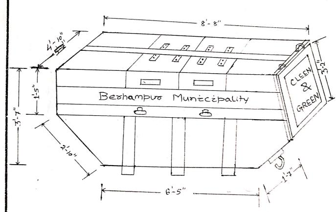
Dumper placer container Buitable to BeMc rehicle.
